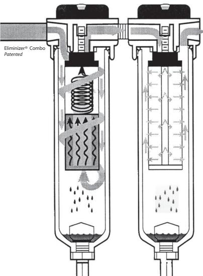
Water-free, Oil-free, Dirt-free Air! 99.99998% efficiency at 0.01 Micron is one of the highest ratings in the industry. Eliminates both water condensates and oil aerosols at point-of-use.
